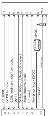
Connects to XIC-1.5 interface cable to XCA radio adaptor
