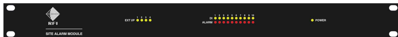
Site Alarm Module (SAM) Front Panel Layout
