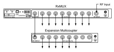
Diagram shows 14 RF Outputs each with a gain of 0 to +15 dB
