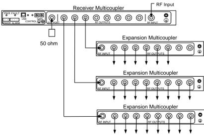
Diagram shows 22 RF Outputs each with a gain of 0 to +5 dB
